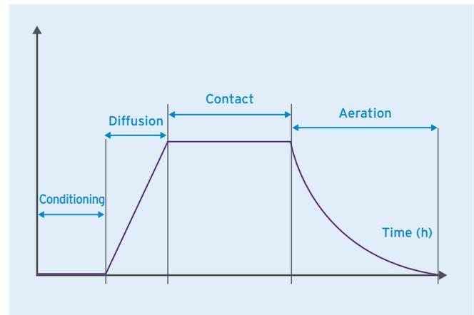
**Conditioning** - where the automated airborne disinfection system and the enclosure to be decontaminated are prepared or conditioned ready for the introduction of the gas, vapour or mist
