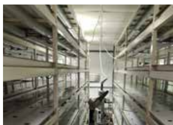
Bioquell RBDS deployed during crop changeover
